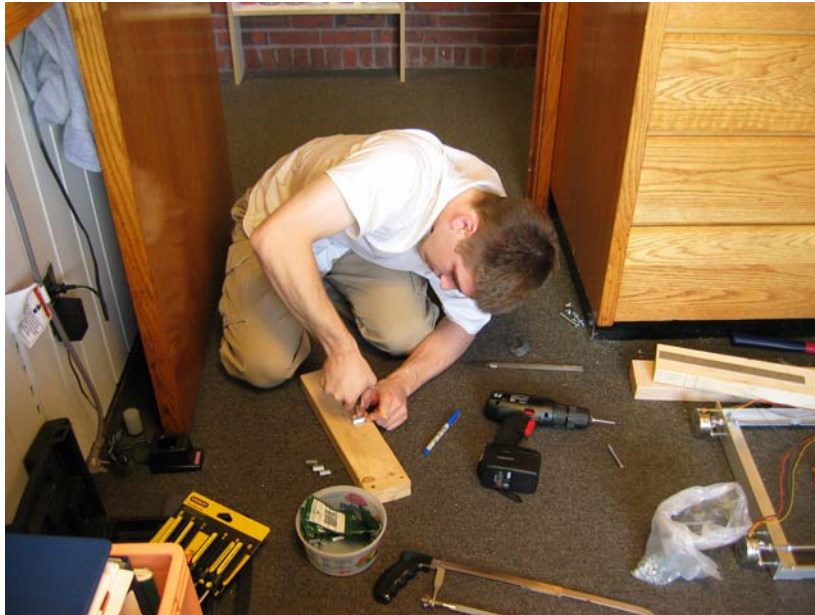
Tapping holes in the hex guide nuts
